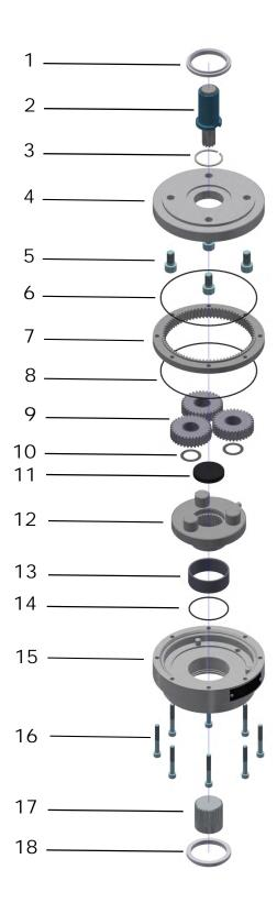
Figure 2: Exploded view QT25, QT50
